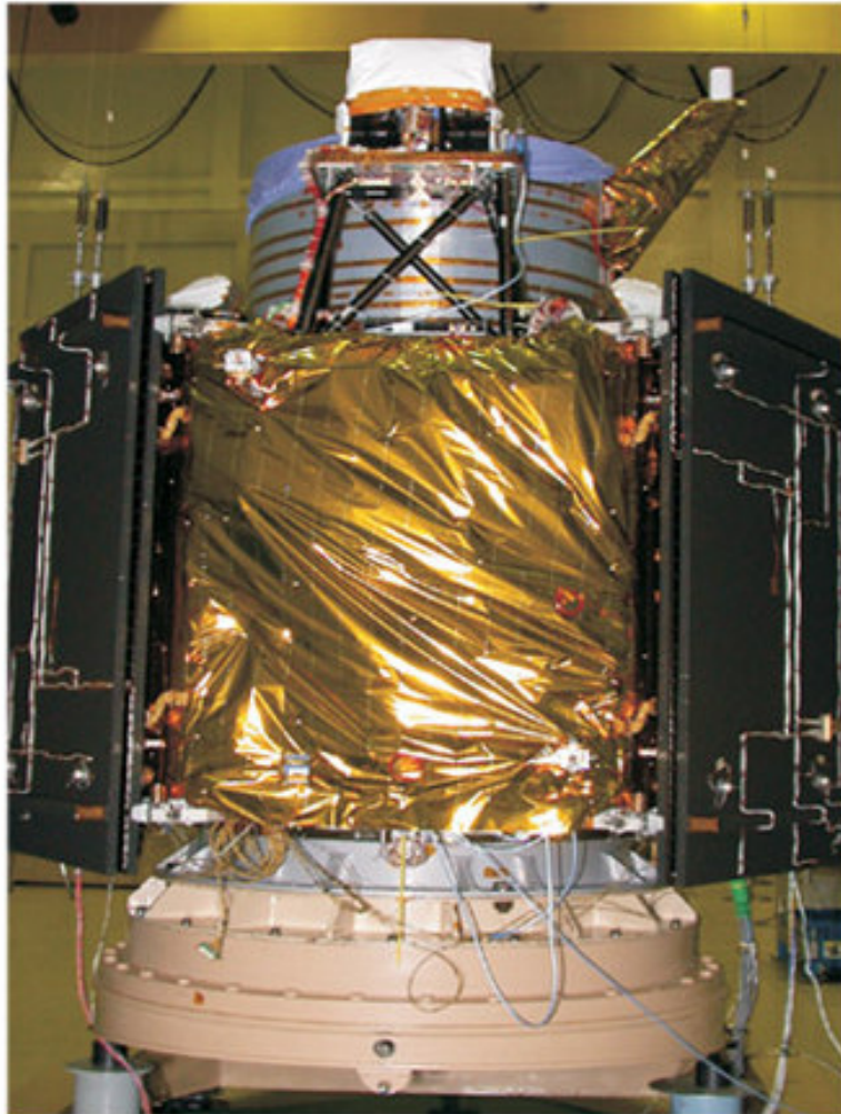
CARTOSAT-2 Spacecraft with its solar panels in stowed condition
